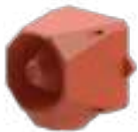
No. 17 851 95 Signal and light alarm for emergency showers. - 112dB(A) output - IP66 protection - 32 alarm tones Working temperature: -20°C to 70°C Power supply: 230VAC, 50/60Hz
